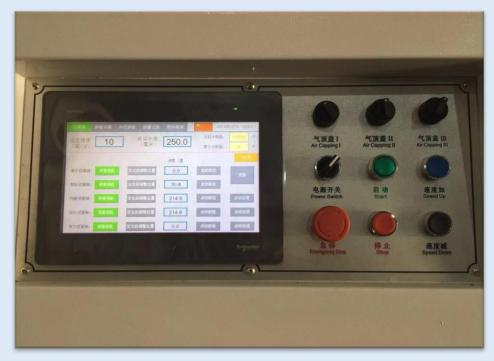
2. The French SCHNEIDER motion controller (PC) is used to ensure stable high-speed operation through the high-speed bus Ether CAT.
